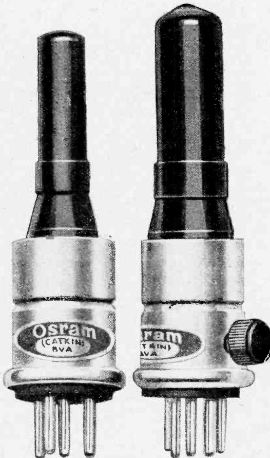
The triode and pentode (unshielded). The rapid cooling of the anode in the case of the pentode gives an increased A.C. watts dissipation.
